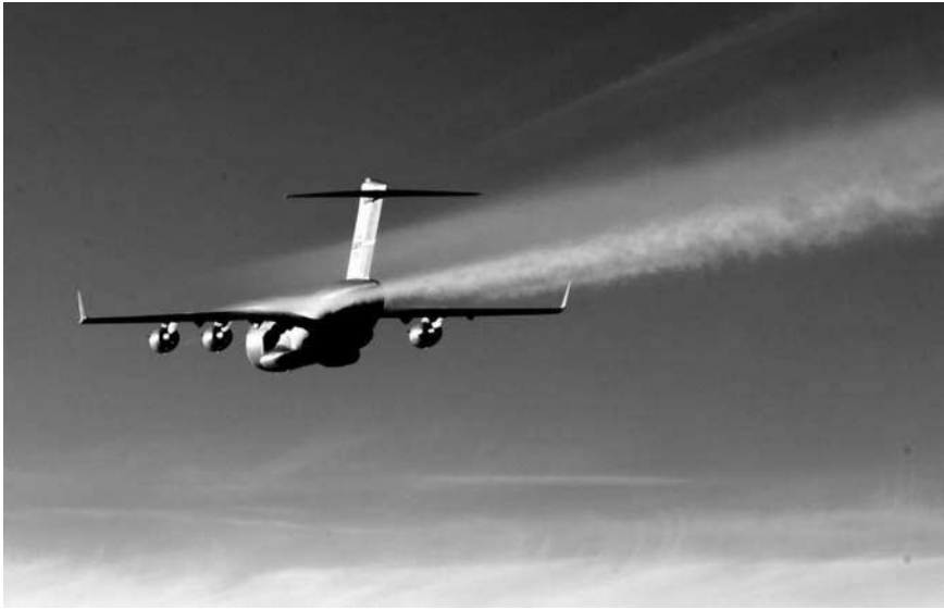
FIGURE 7.3 C-17 Globemaster with wing-mounted nacelles (photo courtesy of the United States Air Force).
