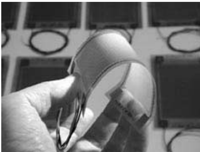
FIGURE 1.11 The Langley Macro-Fiber Composite (LaRC-MFC) is a high performance, low-cost, flexible piezoceramic actuator developed at NASA-Langley Research Center. The solid-state LaRC-MFC is being used to control deflections and vibrations on advanced composite helicopter rotor blades, fixed-wing aircraft control surfaces, and ultralightweight spacecraft components.
