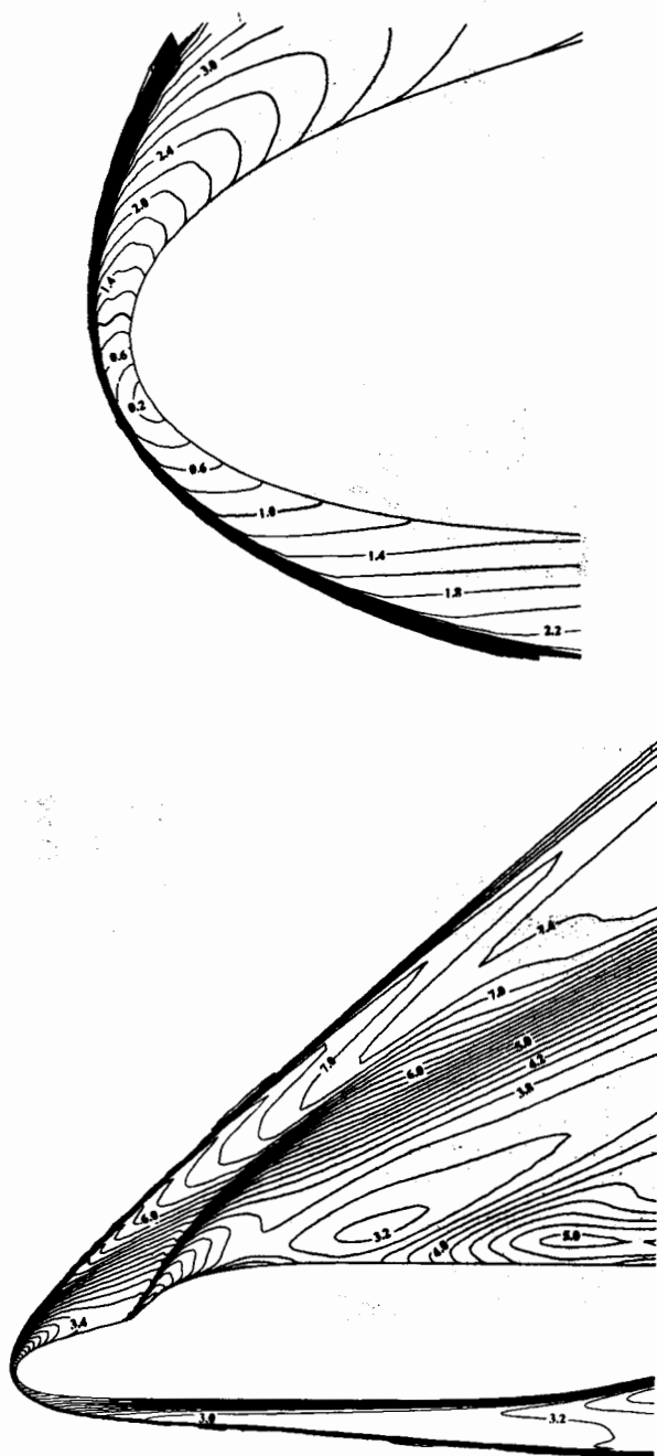
Figure 23.2.9 Mach number distribution in the symmetry plane of the HERMES space shuttle with detailed view of the nose region. (From Rieger and Jameson, 1988. Courtesy H. Rieger, Dornier GmbH)
