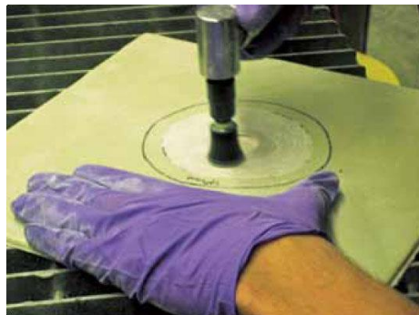
Figure 25. Taper sanding of repair area.
