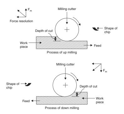
Fig. 4.1 Up and down milling processes
