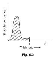
The area under this curve (shown shaded) gives the energy required for the shearing operation.
