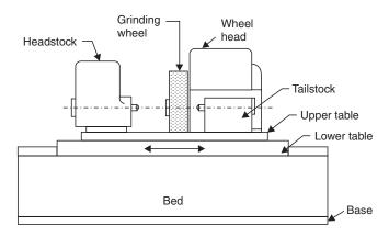
Fig. 5.2 Block diagram of a plain cylindrical grinder
