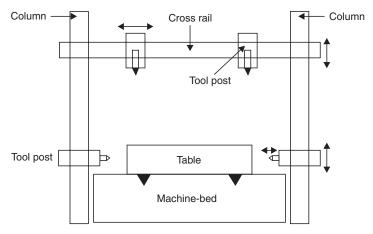
Fig. 2.5 Schematic diagram of a planer
