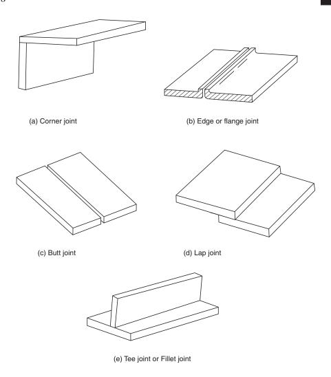
Fig. 6.3 Different types of joints
