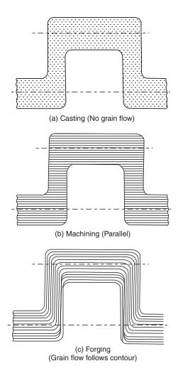
Fig. 1.1 Comparison of grain flow
