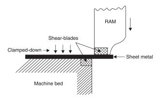
Fig. 5.6 Guillotine shear
