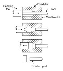
Fig. 2.8 Upset forging on machine
