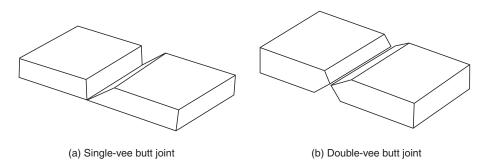
Fig. 6.4 V groove joints
