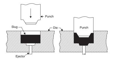
Fig. 4.6 Cold extrusion forging
