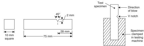
Fig. 1.4 (a) IZOD test specimen
