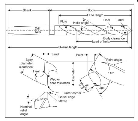
Fig 3.2 Nomenclature of a standard general-purpose twist drill
