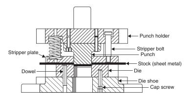
Fig. 5.1 Standard die set with a punch and die mounted in place
