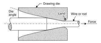
Fig. 4.7 Wire drawing process
