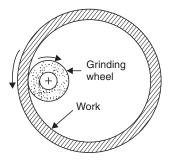
Fig. 5.3 Principle of internal grinding
