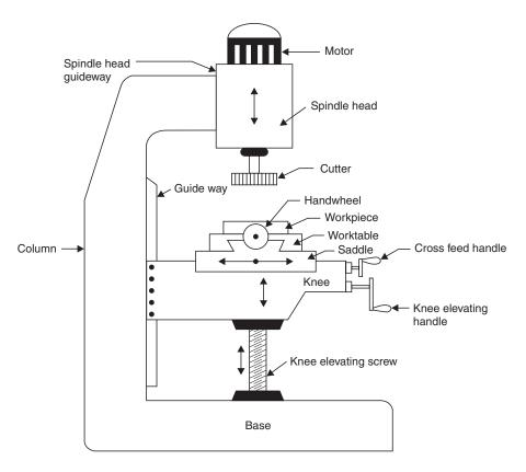
Fig. 4.10 Vertical milling machine
