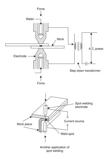
Fig. 6.7 Spot welding process
