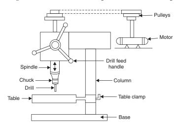
Fig. 3.3 Sensitive or bench drilling machine
