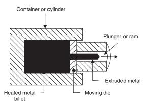
Fig. 4.3 Backward or indirect extrusion
