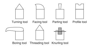
Fig. 1.4 Right hand lathe tools
