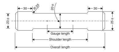
Note: Gauge, shoulder and overall lengths according to IS: 210-1978.
