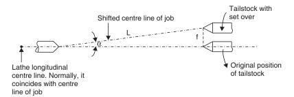
Fig. 1.7 Offsetting tailstock
