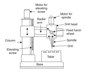
Fig. 3.4 Radial drilling machine
