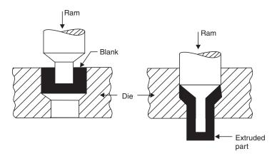
Fig. 4.4 Hooker extrusion
