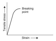
Fig. 1.3 Stress-strain curve for brittle material
