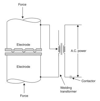
Fig. 6.8 Projection welding
