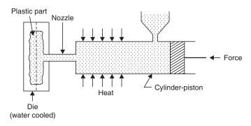
Fig. 4.1 Injection moulding of plastics
