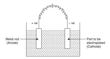
Fig. 4.4 Electroplating process
