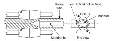
Fig. 4.9 Tube making
