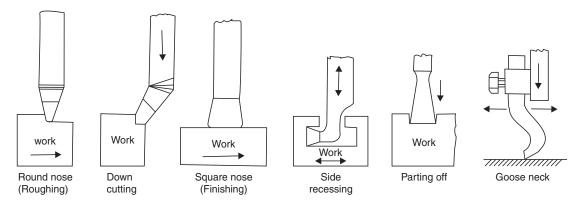
Fig. 2.3 Cutting tools used in shaping work
