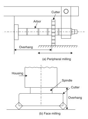
Fig. 4.2 Peripheral and face milling
