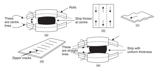
Fig. 3.9 Rolling defects
