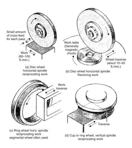
Fig. 5.4 Methods of surface grinding
