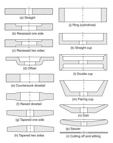
Fig. 5.1 Grinding wheel shapes
