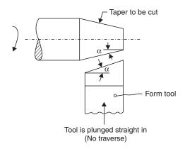
Fig. 1.8 Taper by form tool
