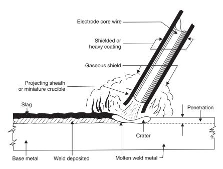
Fig. 6.6 Welding action of a cellulosic-coated stick electrode
