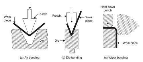
Fig. 5.3 Types of bending dies
