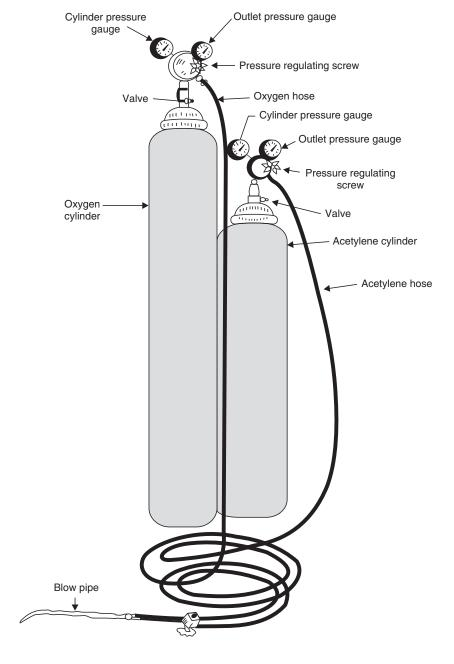
Fig. 6.1 High pressure welding equipment
