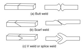
Fig. 2.3 Welded joints and end preparations
