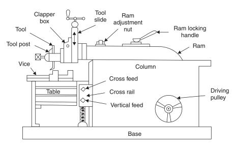
Fig. 2.1 Principal parts of a shaper
