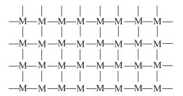
Fig. 3.3 Structure of a thermosetting plastic
