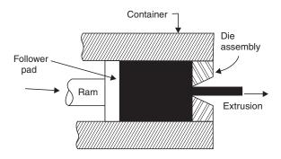
Fig. 4.2 Forward or direct extrusion
