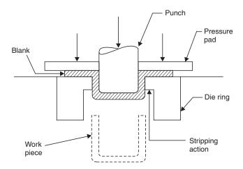
Fig. 5.4 Deep drawing operation
