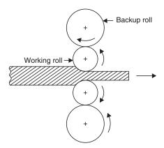
Fig. 3.4 Four high mill
