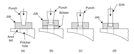
(a) Job placed on anvil and punched half-way on one side (b) Job turned upside down, being punched through using a bolster (c) Job turned upside down, being punched through using Pritchel hole (d) Operation of drifting
