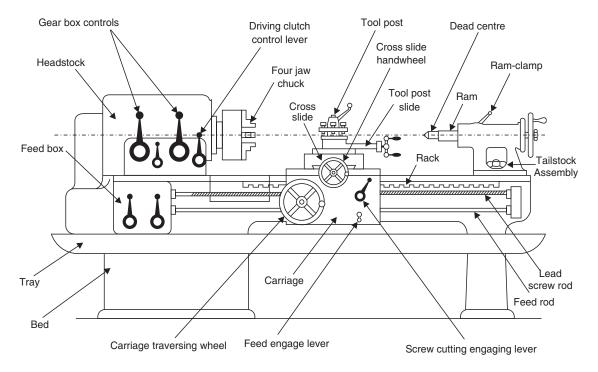
Fig. 1.1 Centre lathe
