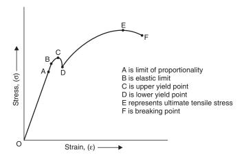
Fig. 1.1 Stress-strain curve for ductile material
