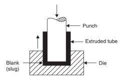
Fig. 4.5 Impact extrusion
