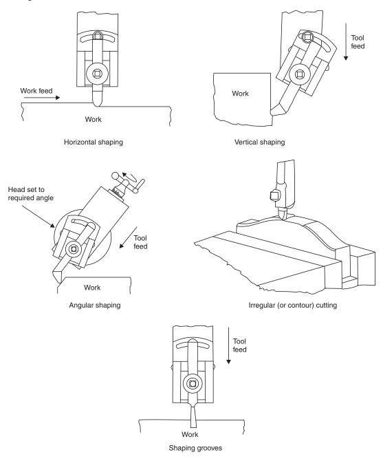
Fig. 2.4 Various operations performed on a shaping machine
