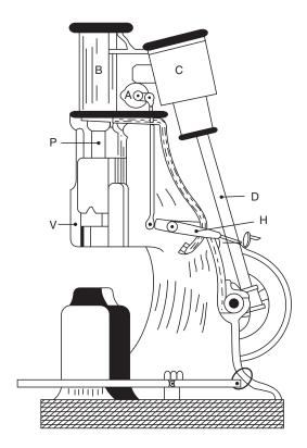
Fig. 2.5 Pneumatic power hammer
