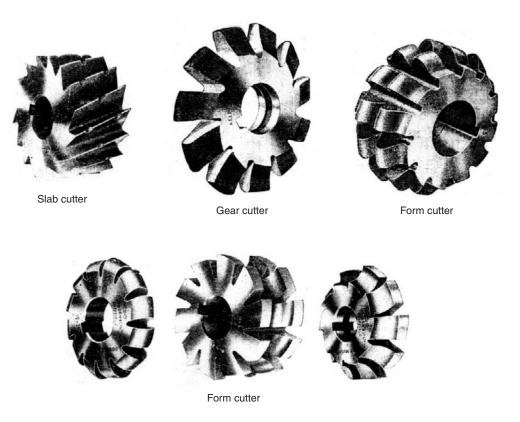
Fig. 4.4 Peripheral milling cutters
