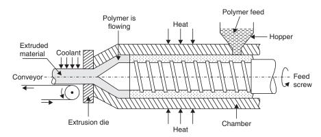
Fig. 4.2 Extrusion of plastics
