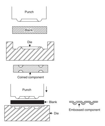
Fig. 5.5 Coining and embossing operations
