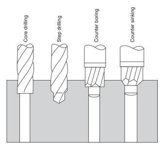
Fig. 3.5 Common operations closely associated with drilling
