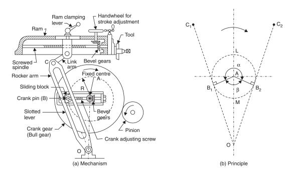
Fig. 2.2 Quick return mechanism
