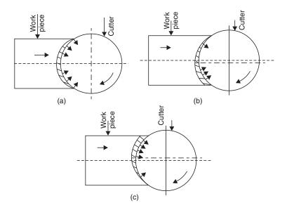
Fig. 4.7 Symmetrical vs asymmetrical milling
