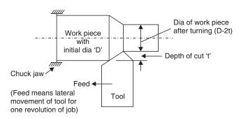
Fig. 1.5 Turning operation
