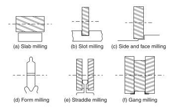
Fig. 4.3 Various peripheral milling operations
