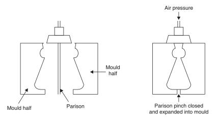
Fig. 4.3 Blow moulding process
