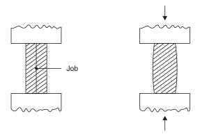
Fig. 2.7 Upsetting with open dies
