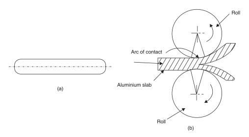
Fig. 3.11 Rolling defect (alligatoring)
