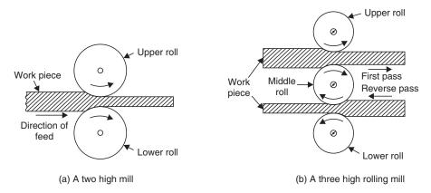
Fig. 3.3 Rolling mill types
