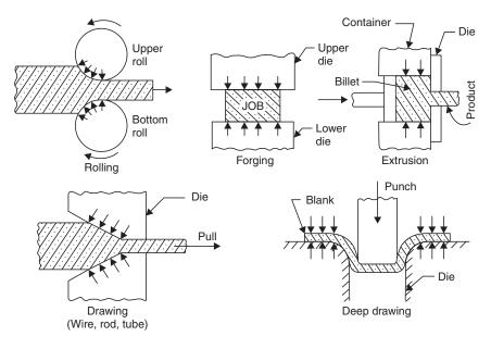
Fig. 1.2 Typical metal working processes
