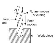
Fig. 3.1 Drilling of a hole
