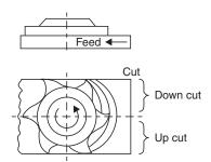
Fig. 4.6 Down and up cut in face milling
