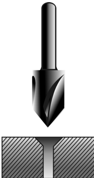
Fig. 4.26, Countersink and countersunk hole.
