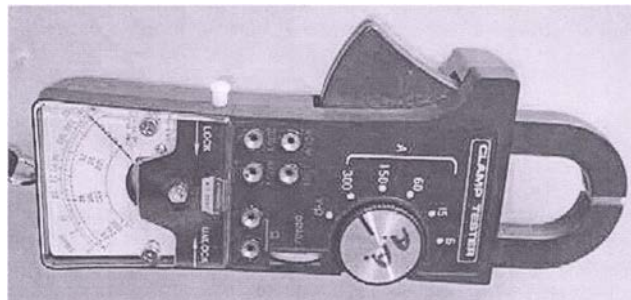
Fig. 10.11, A multimeter with built in clamp
