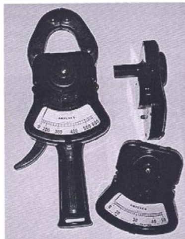
Fig. 10.12, An iron vane type clamp-on ammeter
