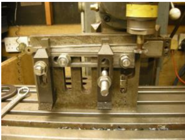
Fig8.5 Machining a connecting rod with a Woodruff cutter
