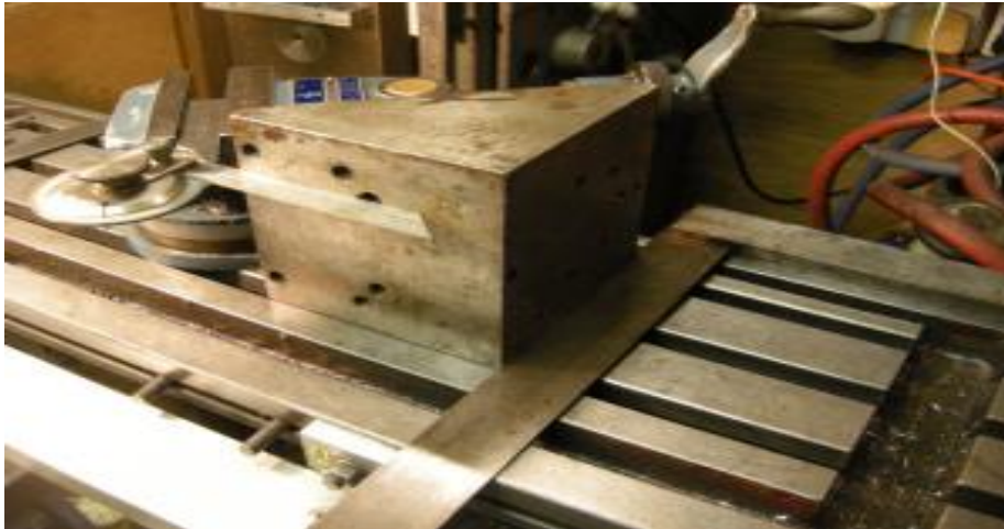
Fig8.3 aligning a vice using a parallel, angle plate and square
