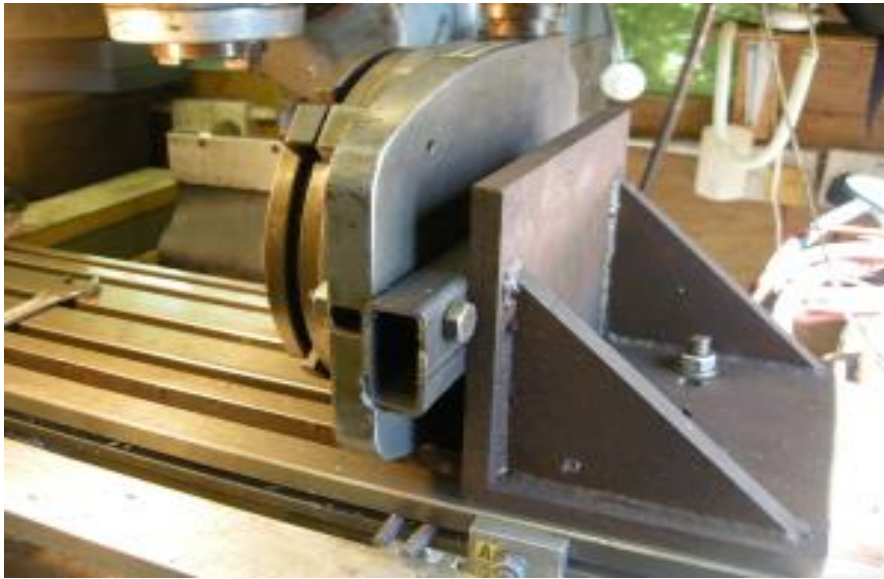
Fig8.2 Rotary table mounted on angle plate using rectangular tube 404
