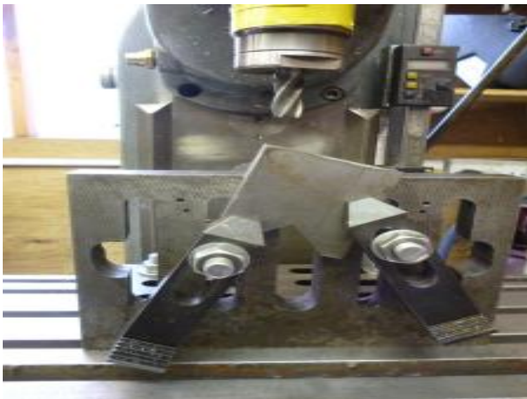
Fig8.4 Machining an edge at an angle
