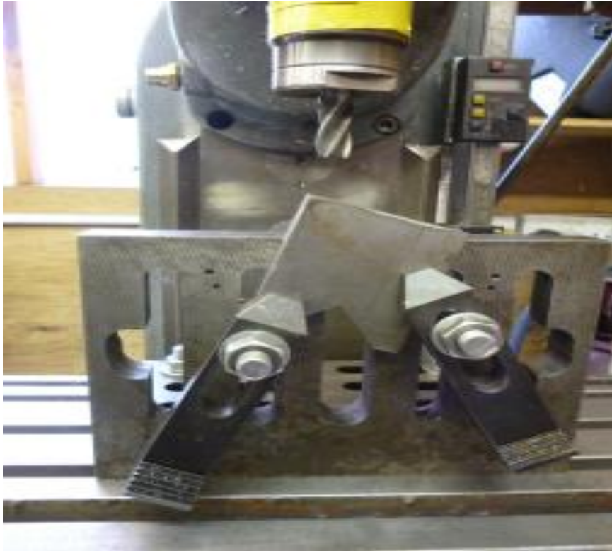
Fig8.1 holding a workpiece on an angle plate to machine its sides
