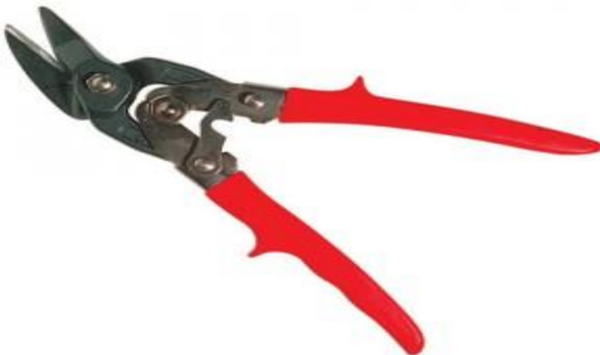
Fig.10.2 Compound action Snipe tool
