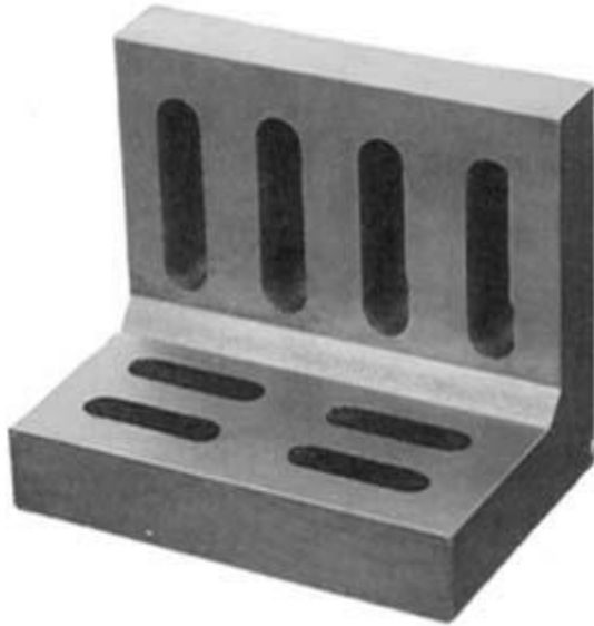
FIG.8.8 Webbed Angle Plate
