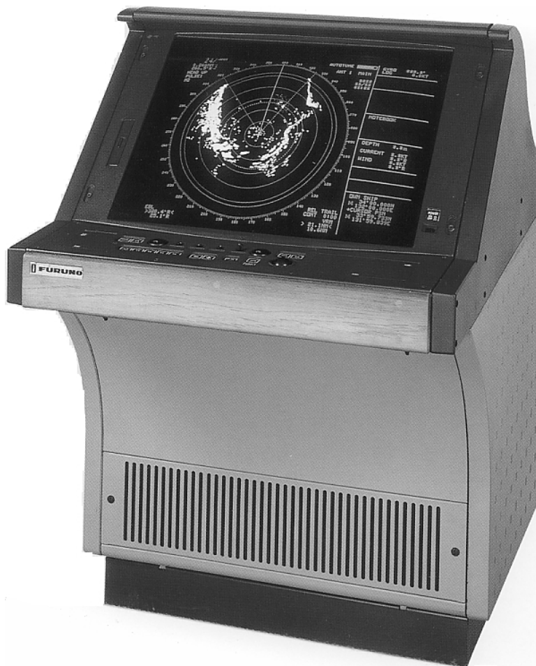
Figure 6.3 Voyager ARPA console. (Reproduced courtesy of Furuno Electric Co. Ltd.)
