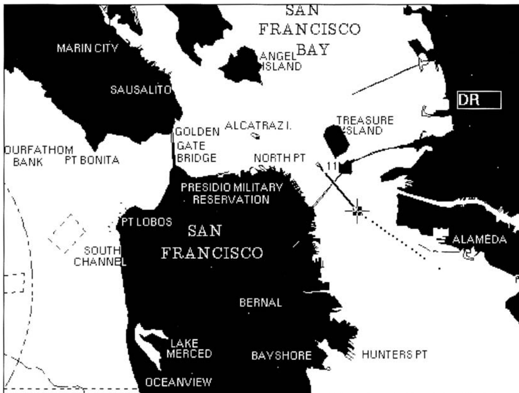
Figure 5.27 Chart display of San Francisco Bay and approaches using data input from a smart card. (Reproduced courtesy of Trimble Navigation Ltd.)
