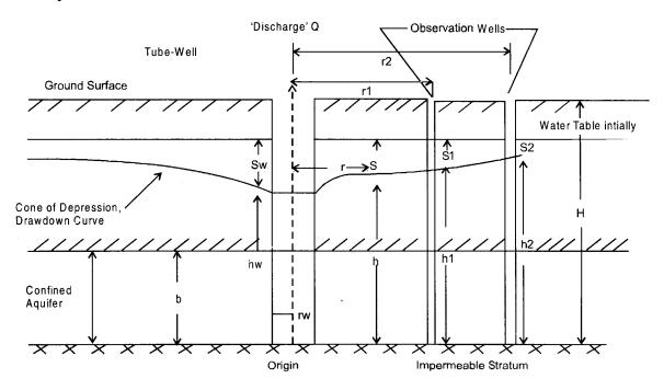
Let us consider the flow through the vertical sides of a cylindrical surface passing through a point P at a distance r. In this case as the depth of the aquifer is only b so the area of flow is equal to  $2 \Pi r b$
