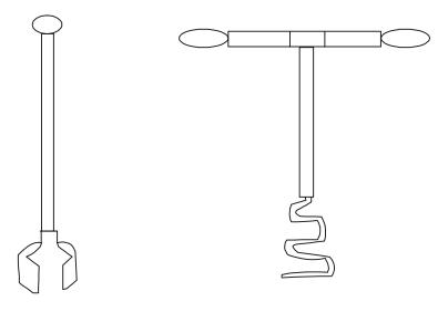
This type of drilling is possible only in soft soils. To support the soft soil casing pipe are lowered simultaneously.
