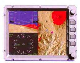
The old "radio stack" will disappear as new and upgraded airplanes, of even the smallest size, are outfitted with EFIS (Electronic Flight Instrument System). This Blue Mountain system combines flight instruments, moving map and terrain warning on one display.
