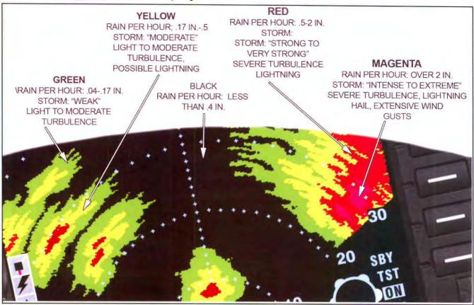
Radar image: Bendix-King The radar image uses five colors to indicate severity of weather; black, green, yellow, red and magenta (a purple-red). The colors are based on the rate of rainfall in inches per hour. Rainfall is also a guide to turbulence in clouds. A pilot may enter the green region, he tries to avoid the yellow, and carefully flies around red and magenta.
