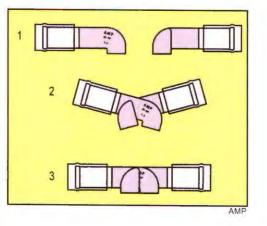
Knife splice is used for quick disconnect.
