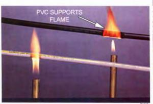
PVC wire was banned by the military, then in commercial aircraft. Besides supporting flame, PVC spreads toxic fumes. Aviation wire is now related to Teflon (left). In photo at right, wire bundles are carefully supported by clamps and cable ties.
