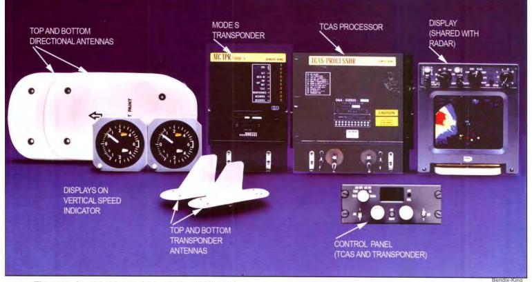
The control panel at lower right selects TCAS and transponder functions. Two antennas are used for the transponder---placed at top and bottom of the fuselage---to assure complete signal coverage around the airplane. Two directional antennas (left) also determine the bearing of a threat aircraft above and below the airplane.
