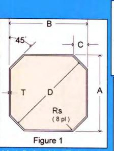
(slanted) edges, it is difficult to make the cut-out with ordinary hand tools. Special cutters are available. Although ATI sizes are an airline
