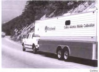
Regulations require that ramp and bench test equipment be calibrated and certified, usually once a year. Many shops send their equipment to calibration laboratories, but another choice is a mobile cal lab. It drives to the shop and performs the work just outside the premises. It also may repair to restore equipment to required accuracy.
