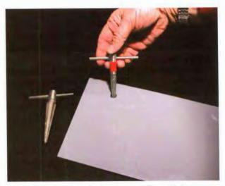
A hand reamer cuts holes in panel for switches, controls and other small items. First, a pilot hole is made with an electric drill.
