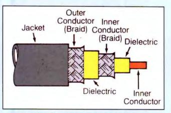
Triaxial cable, with two outer conductors separated by insulation. The outer conductor (braid) serves as a signal ground, while the other is an earth ground. This arrangement provides very high immunity to electrical noise.
