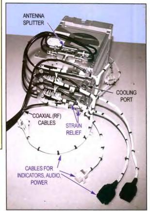
A radio stack, like this one for a light aircraft, is pre-wired on the workbench before installing in the airplane. Three avionics trays are shown; two navcoms on top, with a transponder on the bottom. Wiring is done to connectors mounted on the back of the trays. The radios are slid into place later, and make contact with the rear tray connectors.
