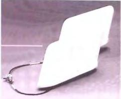
VOR "blade" is a strong, low-drag antenna for turbine-powered aircraft. With a blade on either side of the rudder fin, it is sensitive to VOR ground stations to the left and right of the aircraft course. This improves signals for area navigation (RNAV).
