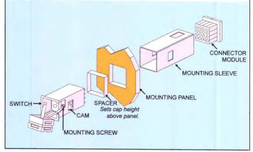
screw and cam. The switch itself may be four independent microswitches, an arrangement which eliminates switch "chatter" during shock and vibration.
