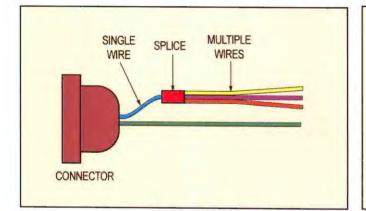
Another exception is when multiple wires need to go to one pin on a connector. They can be spliced to a single wire at the connector.
