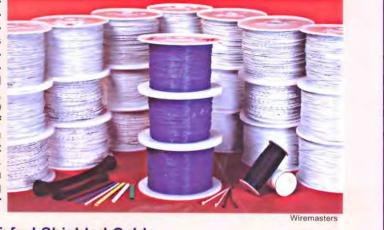
Tin Plated Copper Tefzel Shielded Cable Conductors: 2 Gauge: AWG 22 Shielding: Round Tin coated Copper 85% Min Coverage Jacket: Tefzel Conductor Color Code: White, White/Blue Voltage Rating: 600 Volts Temperature Rating: -55 to +150 Degrees C Weight: 12.40 lbs/Mft Conductor OD: 0.030" Nominal. Outside Diameter Over Finished Cable: 0.124 inch Insulation: ETFE (Ethylene Terafluoroethylene) Mil Spec: MIL-DTL-27500-22TG2T14
