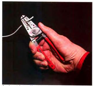
A wire stripper, like this manual type, should have notches to match different wire sizes. A high-quality stripper remains sharp and has a return spring. At the right is a semi-automatic stripper. It grips the wire as blades cut and remove the insulation.
