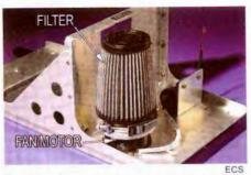
Cooling fan is built into ARINC tray for some airline avionics. A filter removes particles to extend equipment life and raise MTBF (mean time between failure).
