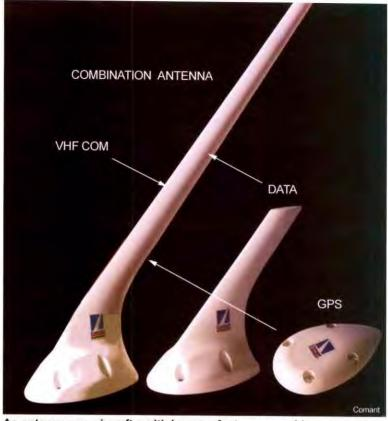
As antennas on aircraft multiply, manufacturers combine several into a single footprint. This example is ComDat; a VHF-com antenna at the left that also contains a GPS or data antenna. The combination not only saves space, it reduces installation time and effort. The antenna has two connectors in the base for attaching cables; a BNCtype for the com radio, and a TNC for GPS or data. The data radio handles such services as weather, messages and traffic information.
