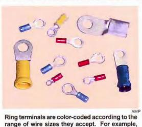
range of wire sizes they accept. For example, red takes any wire from AWG 22 to 16. Also choose the stud size the ring must fit over. For example; the first stud size on the list takes a #4 screw. All ring terminals are crimp-on and self-insulated, except the bare one at top right.
