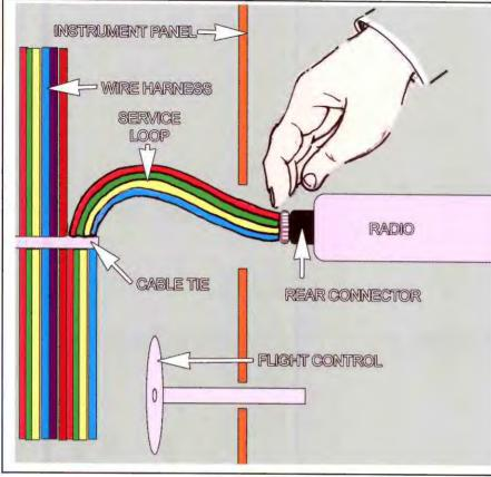
Every radio or instrument should be installed with a "service loop." It is extra slack that permits the radio to slide out of the panel, allowing you to unfasten the connectors. Otherwise, you could spend hours groping behind the panel.
