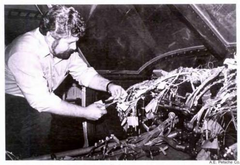
Poor wiring is often called a "rat's nest" but that's not the case in this example. The technician is carefully labelling every wire. Note that all wiring is formed into neat harnesses.
