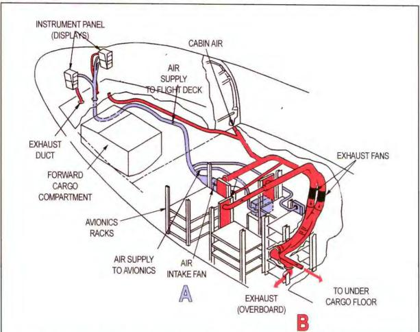
Air transport aircraft have dedicated systems for cooling avionics, as shown in this simplified diagram (based on a B-737). To assure reliability, both sides of the system---intake and exhaust---have two fans each. If one fan fails, an alarm warns the pilot to switch to the alternate.
