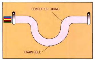
Conduit comes in metal and non-metal versions, rigid and flexible. When selecting a diameter make it about 25% larger than the wire bundle that goes inside. After cutting to length, remove any burrs which might cut the wire. When flexible conduit is cut with a hacksaw, it can have a ragged end. This is avoided by wrapping the end of the conduit with tape before sawing. Conduit also needs to be supported with clamps.
