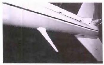
Com antenna on the bottom of a helicopter tail boom. Because of the main and tail rotor blades, antenna locations on helicopters are more difficult to find.
