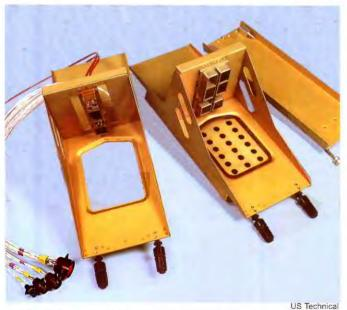
ARINC trays are designed with variations to accommodate different cooling, connector and radio sizes. The black knobs, which lock in the equipment, have a mechanism which cannot be overtightened and damage the connectors.
