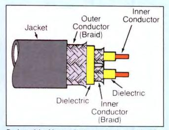
Dual coaxial cable contains two separate coaxial cables covered by a common outer jacket.
