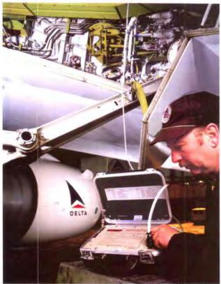
The Model 101A checks autopilot servos and flight control sensors without removing them from the airplane. It measures control voltages to within 5 thousandths of a volt.
