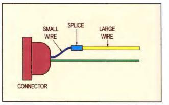
An exception to "one-splice-per-segment" is shown above. If a wire is too large for the connector, splice it to a smaller wire. The small wire from the connector, known as a "pigtail," can be crimped to a connector contact.
