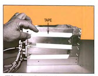
While wiring a radio stack on the workbench, tape the sides of the trays together. This keeps the trays stable while you wire the harnesses at the rear. Remove the tape just before installing the stack in the airplane.
