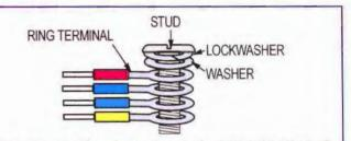
Do not put more than 4 ring terminals under the head of one stud. If more wires must connect, put *three* ring terminals under a stud, plus a *bus bar* (see below). The bar is a short heavy wire or jumper that joins two adjacent studs. This allows three more wires on the second stud, as shown.
