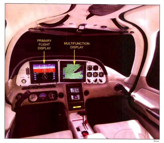
By the year 2000, the future of instrument panels was clear. Flat panels (LCD's) would replace cathode ray tubes (CRT's). Instruments would become "integrated," that is, separate gauges merge into the electronic display.
