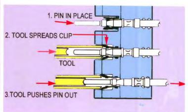
To release pins (1) from a connector, the removal tool is inserted over the pin (2). When the tool seats, it spreads a spring which retains the pin. Now when the tool is pressed further, the pin is pushed (3) out. Shown here is a "front release" connector. Other connectors may be "rear release," but the principle is similar
