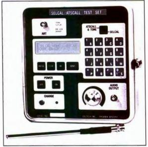
Selective calling systems aboard aircraft are checked remotely by this ramp tester, the Avtech CTS-700. It sends and receives the 16-tone code of the ARINC Selcal system. It also communicates with Atscall, a system used in some fleets, which is based on the 16 "touchtone" codes used in telephone systems. As in many ramp testers, battery power is automatically turned off if there is no activity for 15 minutes.
