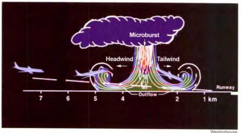
Wind shear---a sudden change in wind direction or speed---is most hazardous when the aircraft is close to the ground, as during an approach. Windshear mostly affects pure jet aircraft because of slow turbine "spool-up" time; a delay of about 4 to 7 seconds after the pilot calls for full power.
