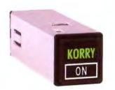
Improved lighted pushbutton switches, like this Korry model, eliminate a major source of maintenance; replacing lamps with burned-out filaments. Lighting is supplied by bright LED's (light emitting diodes) that can last the life of the airplane. They also run cooler than conventional lamps.
