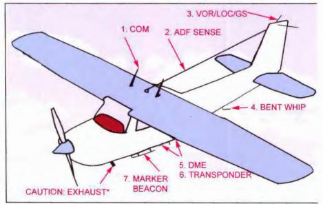
Don't locate an antenna on the belly in line with an exhaust pipe. It becomes coated and discolored. Locate antennas as close as possible to the centerline of the fuselage, but avoid cutting into structure like ribs and stringers. resistance electrical ground to the airframe---all factors covered in this chapter.
