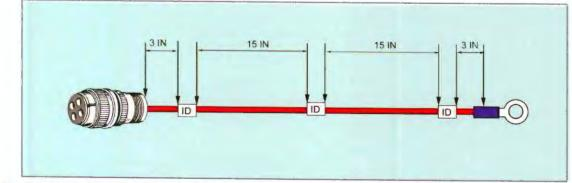
Individual wires should be marked. The recommended spacing is an identification ("ID") marker within three inches of where the wire originates (in this example, a connector, and within three inches of where it ends at the ring terminal at the right). Along the wiring run a marker should be installed at a maximum of every six feet. Wires less than three inches long require no ID. Wires between three and seven inches should be marked at about the center.
