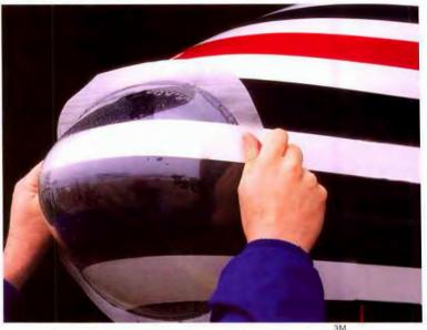
A pre-formed boot made of polyurethane may be applied over the radome for added protection. It reduces the effects of rain, snow, sleet, insects, sand and ultraviolet light
