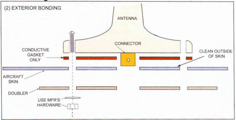
In the exterior method, bonding is made to the outside skin. Thus, the skin must be cleaned and treated with Alodyne to prevent corrosion. Only a *conductive* gasket can be used with exterior bonding; there must be good electrical contact with the outer skin.
