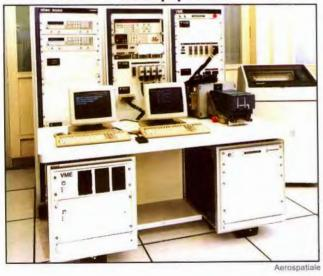
Automatic Test Equipment (ATE), like this ATEC 5000, checks digital circuits in airliners and military aircraft. It contains programs that automatically test hundreds of parameters. To locate intermittent problems, the test station runs continuously until a fault appears. The time and location of the fault are stored for later viewing by the technician. ATE systems like these are usually found at large airline and repair depots.
