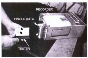
When testing the underwater locator beacon (the "pinger") the tone is ultrasonic and cannot be heard by the ear. The tester receives the tone and converts it down to the range of human hearing. To start the pinger operating, one end is moistened to simulate an underwater condition.
