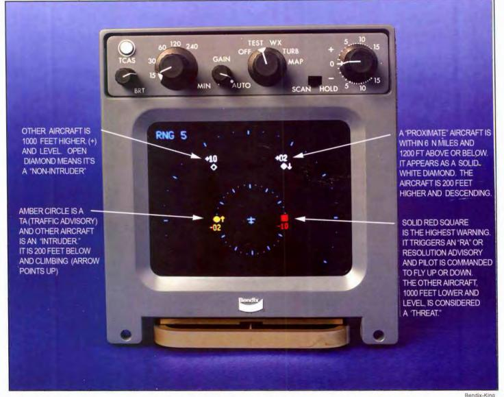
If an airplane has an EFIS or radar display, it can show TCAS information. The weather radar control panel is at the top, with a button at top left for activating the TCAS display.
