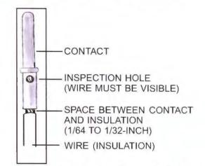
In this type of contact, there is an inspection hole. Bare wire must be visible through the hole. There must also be a small space between the contact and the insulation.
