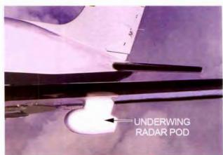
Radar antenna for a single-engine airplane cannot mount in the nose because of the propellor. Instead, it is located under the wing, as shown above, or built into the leading edge of wing.
