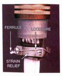
Strain relief for cable is provided by clamp at back of connector. Screws are secured by safety wire applied by tool. (Illustrations: DMC)
