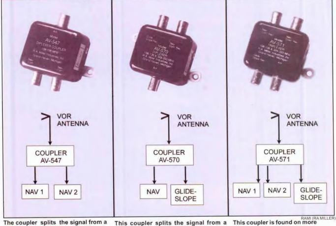
The coupler splits the signal from a single antenna to feed two VOR navigation receivers. As in most couplers, it is only for receivers, which operate on very low-level signals. All couplers reduce the antenna signal by splitting, but there is ample signal strength remaining to do the job.
