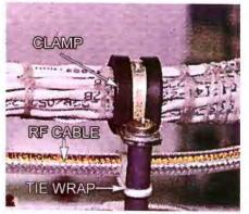
The large wire bundle at the top is supported by a clamp. Wires contained in the bundle carry low-level signals (receiver, data, control, audio, etc.) that don't interfere with each other.
