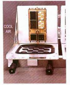
Holes in bottom of ARINC-type tray admit air to cool avionics.
