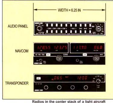
Radios in the center stack of a light aircraft are usually 6.25 inches wide.
