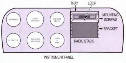
Although panel-mount radios are associated with small aircraft, they're also found in commercial aircraft (commuter and regional airlines). The panel mount uses the instrument panel as the support structure. A rectangular hole is cut in the panel and vertical brackets riveted to the sides of the opening. The tray (which receives the radio) is bolted to the brackets. After the tray is mounted, the radio is slid in and locked by turning a front panel screw, as shown.
