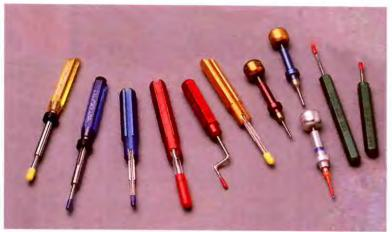
A variety of tools is available for installing and removing connector pins, either front or rear release. Although these tools may be offered in plastic, metal is preferred for durability.
