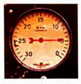
Tachometer from a 1931 Piper Cub is a 3-inch instrument that shows one function: RPM.
