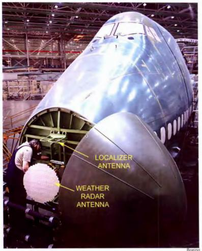
can reach (or crawl) inside the airplane to the area of the antenna base. You may need to install a doubler plate, attach an antenna connector or install strain relief for the cable from inside the airplane.
