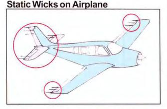
Typical locations are shown for static wicks on trailing edges of wings and tail. Manufacturers of wicks provide drawings for most aircraft that show exact locations.
