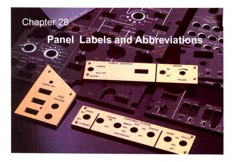
According to regulation, all controls and indicators on an airplane must be clearly labelled and visible to the pilot. Unmarked items can be handled several ways:
