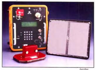
The IFF-701 is a flightline transponder tester. It performs single checks or an autotest that runs 30 tests automatically. The tester communicates with the aircraft through its antenna. The red object at the lower left is an antenna shield, which covers one aircraft antenna in installations where there are two transponders (in an anti-collision, or TCAS, system).
