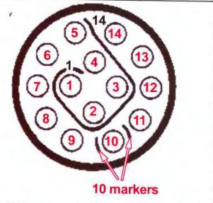
2. The same connector is shown; with red numbers added to clarify the numbering system. Note that "10" is surrounded by two markers. They speed up your counting. You can jump to the first marker and know it's 10. When looking at the back of a connector (where the terminals are inserted or wired) counting is usually done in a counterclockwise direction.
