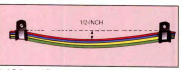
Install clamps at distances no more than 24 inches apart. When you grab the wire bundle and give it a *slight* pull, it should not move axially (to the left or right in this illustration). The bundle may droop up to 1/2-inch under normal conditions. That slack may be exceeded if you are sure the bundle cannot touch a nearby surface and suffer damage from abrasion (rubbing).
