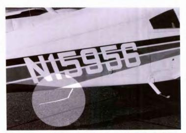
When a com antenna must be mounted on the belly of a light aircraft, use a "bent whip" to prevent striking the ground. Although not as efficient as a top-mounted antenna, the bent whip shown here was used for 10 years. It reliably communicated 50 miles in every direction at an altitude of 3000 feet,
