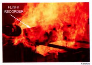
Manufacturers of flight data recorders must comply with standards for survivability in a crash. A recorder should withstand a temperature of 1100 degrees C for 30 minutes, as shown in this test. In another test, a 500-pound weight is dropped on the recorder from 10 feet.
