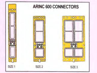
ARINC 600 appeared with the new generation of "digital" airliners during the 1980's, including the Boeing-757, -767 and Airbus A-320. Because of the advanced systems, ARINC 600 provides more contacts in a small area
