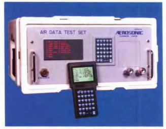
Air data test set by Aerosonic. It checks altimeter, encoding altimeter, airspeed, Mach airspeed, rate-of-climb and cabin pressure. The hand-held remote (at the bottom) enables the technician to sit in the cockpit and observe the instruments while operating the tester located elsewhere. Operating limits can be set to avoid delivering excess pressure to the instruments.
