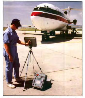
Tests to verify and certify a TCAS (Traffic Alert and Collision Avoidance System) can be done outside the airplane. The ramp tester, an Aeroflex TCAS-201, communicates with the airplane via radio signals and simulates different collision conditions. Without connecting directly into airplane systems it measures signal power, frequency, interrogations and replies. The tester is programmable to perform ten different collision scenarios.
