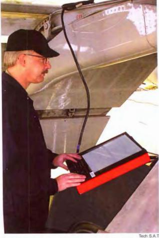
Flightline portable test set loads software on airplane through port in wheel well. It also contains fault diagnostics and flight data analysis. The tester's operating system is Windows-based.
