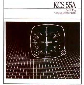
Typical manufacturer's manual for General Aviation, in this illustration a Bendix-King compass system with a horizontal situation indicator. Always check the model number on the unit and compare it with the manual. For example, the model name "KCS 55A" may not be the same as "KC 55," although the illustration may appear the same.
