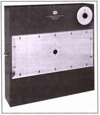
This test box measures loop and sense antennas of an ADF receiver. The antenna is mounted inside the box and stimulated by test signals. A 10-inch dial on the simulator is rotated to measure bearing within a 1/2-degree over 360 degrees. These tests once required a shielded room. The tester shown here is the TIC CES-117A.
