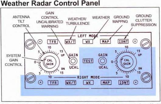
Both the captain and first officer operate the weather radar from the same control panel in this ARINC-type unit. Nearly all controls are duplicated; the captain's side is the white area, the copilot's is shown with a blue background. They are grouped as ""Left Mode" and "Right Mode" to indicate that the controls affect left and right sides of the instrument panel.
