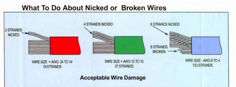
If you accidently nick or break a strand of wire, you may be able to install it anyway by following FAA guidelines shown above. Determine the number of strands in the wire (a figure usually available from the supplier, or simply count them). As shown in the first example, at the left, there can be two nicked strands in wires from AWG 24 to 14, so long as all other strands are in tact. Broken wires are allowed in larger wires at the right, which can contain 133 strands.
