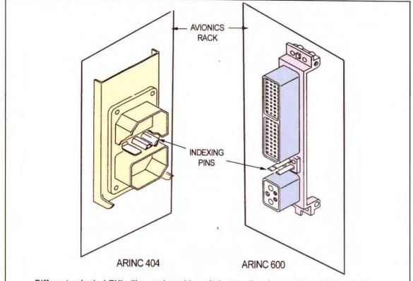
Different avionic LRU's (line replaceable units) are often housed in cabinets of the same size---which could cause installation error. To prevent it, a connector has an indexing pin at an angle that matches only one LRU. Unless all pins line up with connector holes, the radio cannot be pushed in. To prevent damage, however, avoid forcing a radio into the rack.
