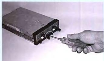
A panel-mounted radio is removed from the instrument panel by inserting a tool into an opening on the front. It may be a screwdriver, hex wrench or other tool.
