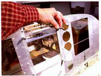
In this construction of a new instrument panel, radio trays are being riveted to brackets. The brackets were fastened earlier to the panel.
