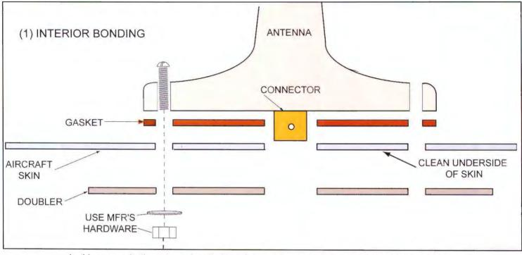
In this approach, the antenna bonds through its mounting screws to the aircraft skin *inside* the fuselage. The inside area, therefore, must be clean and corrosion-free. After clean-up, apply Alodine to the bare skin to slow future corrosion.
