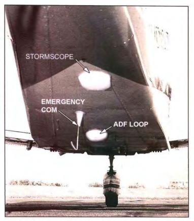
Belly of a single-engine aircraft. Stormscope antenna is for weather (lightning) detection. The ADF loop is forward. Between them is a "bent-whip" com antenna to connect a handietalkie during radio or electrical failure. Some pilots also use it to listen for clearances while waiting on the ground with the engine off.
