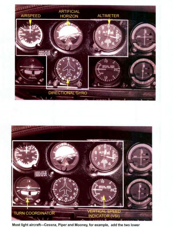
Most light aircraft---Cessna, Piper and Mooney, for example, add the two lower instruments to the basic T; the turn coordinator and vertical speed indicator. This equips the airplane for basic instrument flying. Some technicians call this the "six pack."
