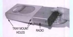
Radio is shown sliding into mounting tray. Holes in the tray are for fastening the tray to the instrument panel.
