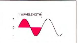
A radio signal can be pictured as an alternating flow (the shape of a sine wave). Electrical energy for the first cycle begins from zero (at left) and rises in strength in the positive direction. Next, it drops to zero, reverses and strengthens in the negative direction. This completes one cycle, measured in Hertz (Hz). If the cycle repeats 122 million times per second, the frequency is 122 MHz (megahertz), which falls in the aviation com band.
