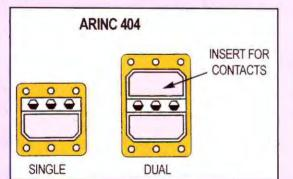
ARINC 404 is aboard airliners that began production during the 1960's. This includes first models of the Boeing-727, -737, -747 and Airbus-300. Instruments and radios operate on conventional (analog) principles, which require fewer pins than today's avionics. These connectors are set up for various equipment by different inserts (which hold the contacts). The ARINC 404 connector is still needed on most recent airliners.
