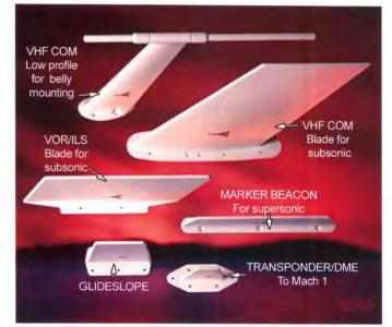
Antennas by HR Smith for high-performance aircraft are encased in thermosplastic composite material to resist rain erosion, impact, chemicals and temperature changes.
