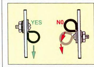
When mounting cable clamps on a vertical surface, locate the nut and bolt *above* the loop that holds the wire (see "Yes"). Placing them below, as shown at "No," may cause wiring to sag if the hardware loosens. This could cause trouble.
