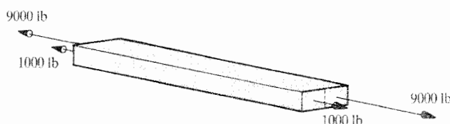
Figure 1.2. Illustration of the possibility of a nonuniform distribution of axial stresses across the cross-section of a bar.
