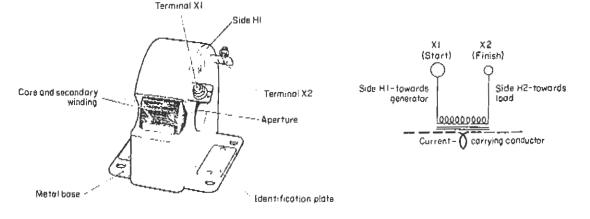
Fig 3.12 Current transformer
