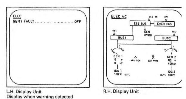
Fig 8.15 Display in failure-related mode
