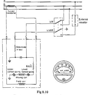
Circuit arrangements of a watt/VAR meter
