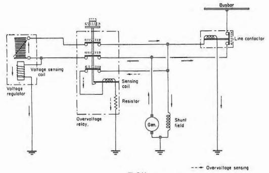
Fig 7.11 Overvoltage protection d.c. generating system
