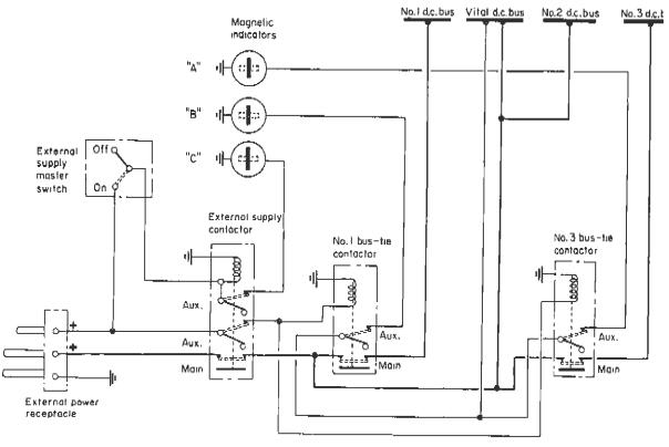
Fig 4.5 Schematic of an external power supply - multiple d.c. busbar system
