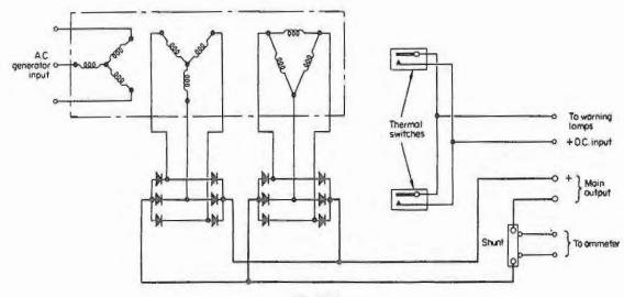
Fig 3.17 Schematic circuit of a transformer-rectifier unit
