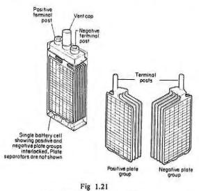
Typical lead-acid secondary cell
