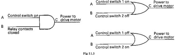
Fig 11.5 Logic gate/theoretical circuit relationship
