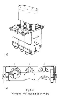
(usually to a "system off" position). This is accomplished by a separate gang-bar mounted on the control panel in such a way that it can be pulled down to bear against the toggles of the switches to push them in the required direction. When the bar is released it is returned under the action of a spring.
