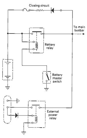
Fig.1.31 Battery charging from external power
