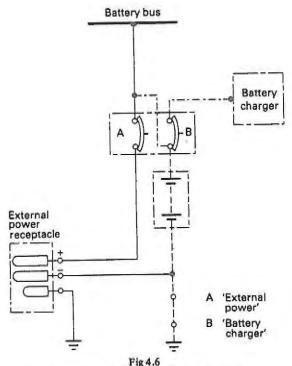
Separate external d.c. supply for A.P.U. starting
