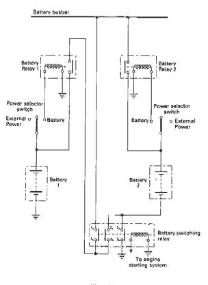
Fig 1.30 Parallel/series connection of batteries
