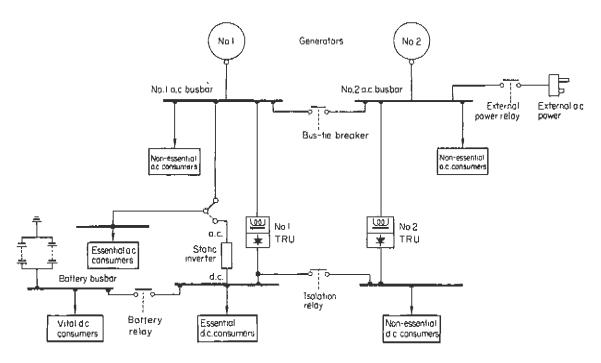
Fig 5.2 Split busbar system (primary a.c. power source)
