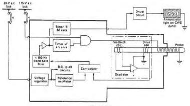
Fig 10.30 Functional diagram of ultrasonic probe system
