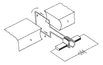
Fig 9.1 D.C. motor principle
