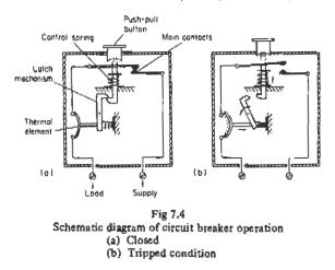
the circuit breaker is shown in its normal operating position; current passes through the switch unit contacts and the thermal element, which thus carries the
