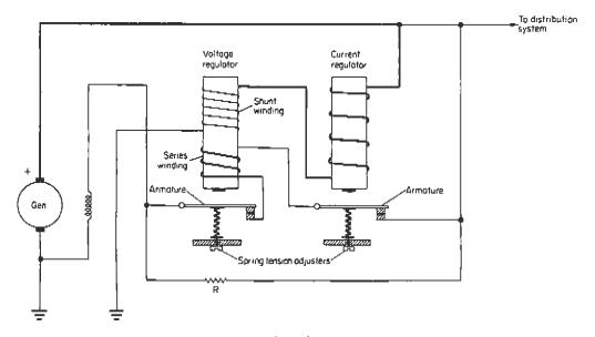
Fig 1.13 Vibrating contact regulator principle
