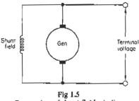
Connection of shunt-field winding
