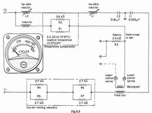
Circuit arrangements of a frequency meter
