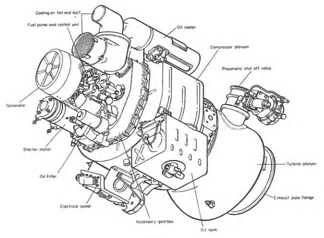
Fig 4.9 Auxiliary power unit
