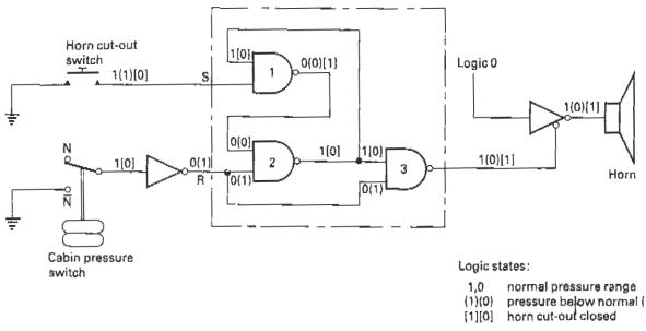
Fig 11.10 Logic diagram of a low-pressure warning system
