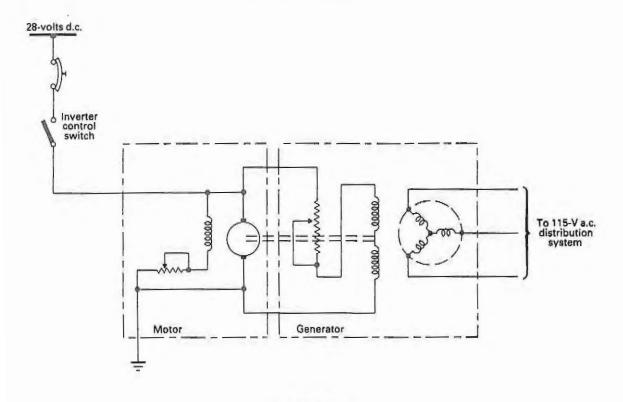
Fig 3.18 Rotary inverter operation
