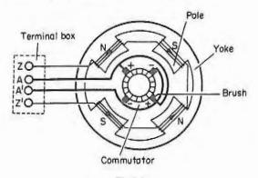
Fig 1.4 Fixed winding arrangements
