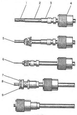
Fig 5.10 Typical coaxial cable and end fitting 1. Outer braid conductor 2. Outer covering
