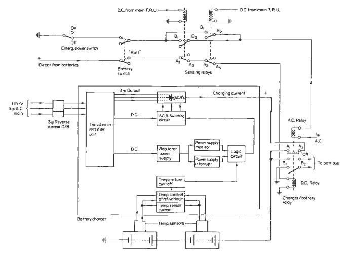
Fig 1.32 In-situ battery charging system
