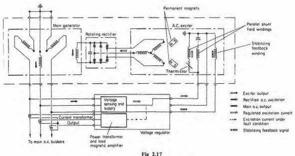
Circuit diagram of constant frequency generator
