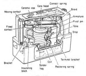
Fig 6.15 Attracted armature relay (unsealed type)
