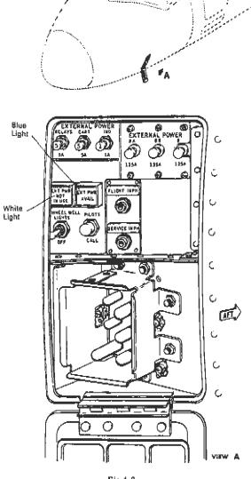
Fig 4.8 External a.c. power receptacle and control panel not supplying power to any a.c. load husbar on the aircraft. The blue light is illuminated whenever a.c. power is being supplied to the load husbars.
