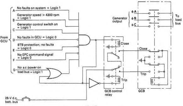
Fig 11.9 Logic diagram – generator circuit breaker control
