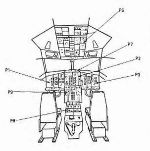
Fig 5.19 Flight deck control panels
