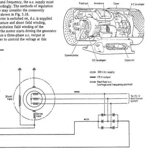
Fig 3.19 Rotary inverter (carbon-pile regulation)
