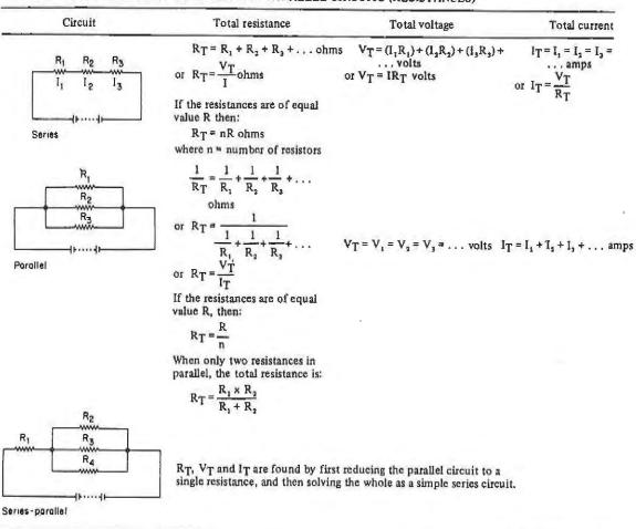
APPLICATION OF OHM'S LAW TO SERIES AND PARALLEL CIRCUITS (RESISTANCES)
