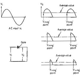
Fig. 3.6 Variable d.c. output from a silicon controlled rectifier
