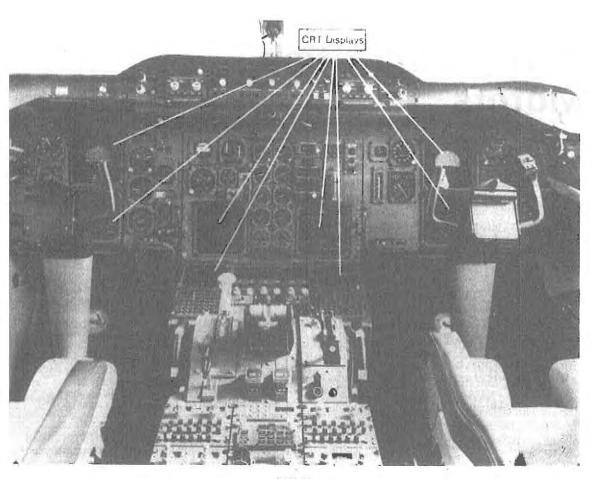
Fig 8.16 CRT display unit locations (Airbus A310)
