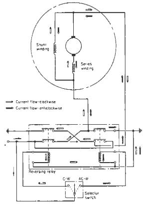
Fig 9.6 Reversing of a compound motor
