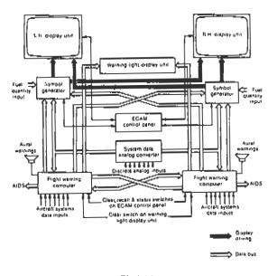
Fig 8.14 Schematic functional diagram -- ECAM system
