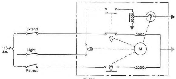
Fig 10.6 Extending/retracting light circuit
