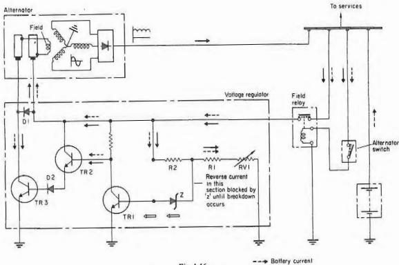
Fig 1.16 Solid-state voltage regulator
