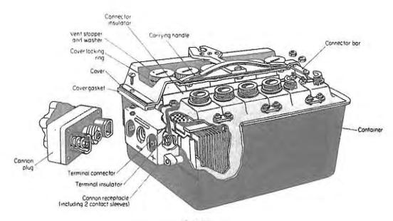
Fig 1.23 Lead-acid battery (absorbed liquid type)
