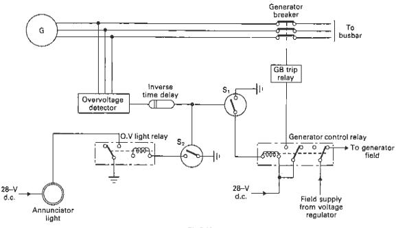
Fig 7.13 Overvoltage protection (constant frequency system)
