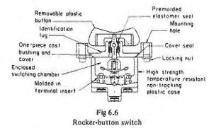
central spindle carrying one or more contact plates or blades which engage with corresponding fixed contacts mounted on the switch base. The movement is usually spring-loaded and equipped with some form of eccentric device to give a snap action and positive engagement of the contact surfaces.
