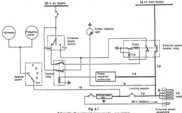
Schematic of an external power supply - a.c. system
