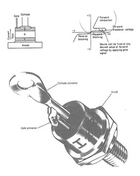
Fig 3.5 Silicon controlled rectifier
