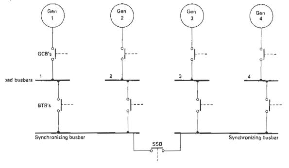
Fig 5.5 Combinations of parallel operation
