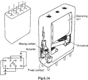
Attracted armature light-duty relay (scaled)
