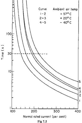
Characteristic curves of a typical circuit breaker tripping times
