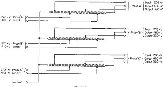
Fig 3.15 Tappings of a typical three-phase auto-transformer
