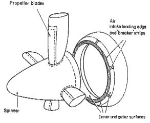
Fig 10.23 Propeller and air intake de-icing system
