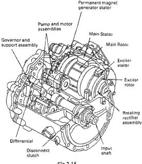
Fig 2.15 Integrated drive generator
