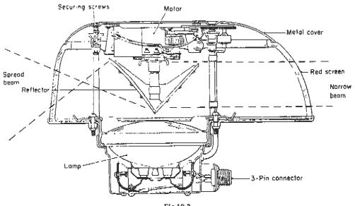
Fig 10.2 Rotating reflector beacon
