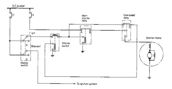
Fig 10.12 Basic circuit of a turboprop engine starting system
