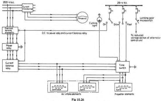
Engine air intake and propeller de-icing and anti-icing control circuit
