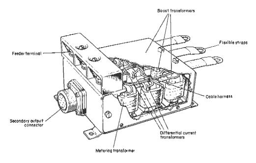
Fig 3.13 Current transformer package
