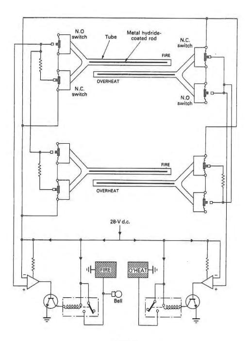
Fig 10.18 Overheat and fire detection system
