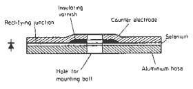
Fig 3.2 Cross-section of a selenium rectifier element
