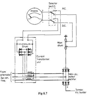
Measurement of d.c. loads in a rectified a.c. system
