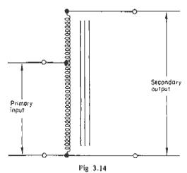
Circuit arrangement of an auto-transformer
