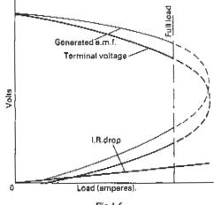
Fig 1.6 Characteristic of self-excited shunt-wound generator
