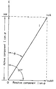
Fig 2.6 Components of current due to phase difference
