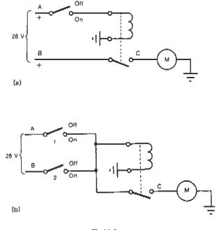
Fig 11.2 Logic switching functions
