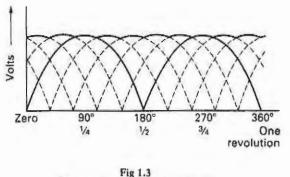
Effect on output using several coils
