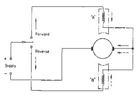
Fig 9.5 Split field motor circuit
