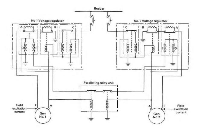
Fig 1.20 Load sharing (vibrating contact regulators)
