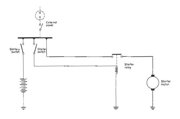
Fig 10.11 Simple engine starting system
