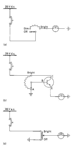
Fig 10.10 Control of lighting intensity
