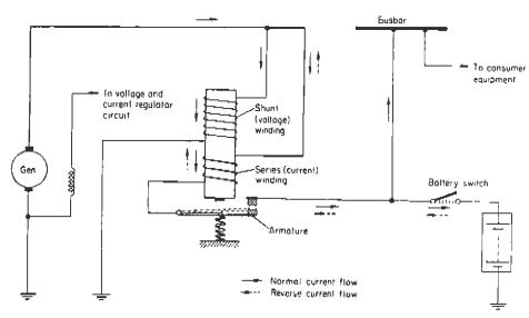
Fig 7.7 Reverse current cut-out operation
