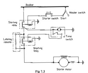
Application of a limiting resistor
