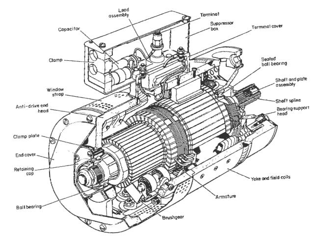
Fig 1.7 Sectioned view of a generator
