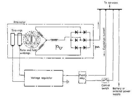
Fig 1.9 Circuit diagram of alternator
