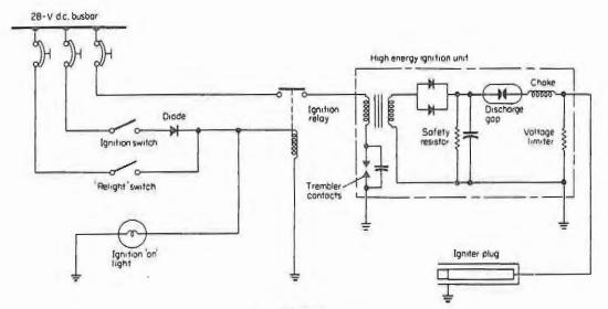
Fig 10.14 High-energy ignition system
