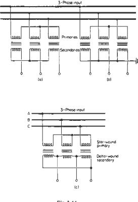
Fig 3.11 Circuit connections for three-phase transformers (a) Star connection three-wire (b) Star connection four-wire (c) Star and Délta connection
