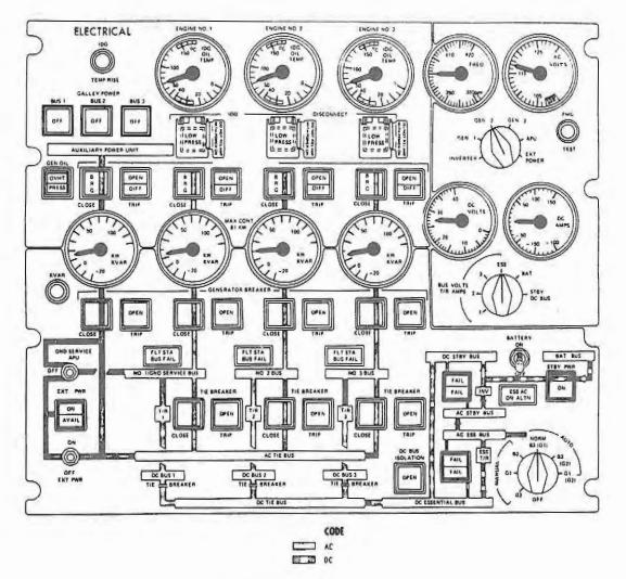
Fig 8.1 Electrical system control panel
