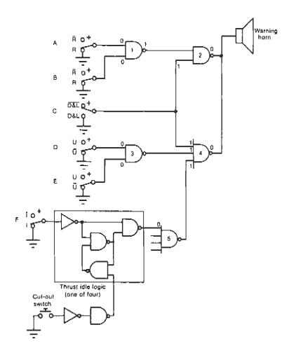
Fig 11.11 Logic diagram of a landing-gear aural warning system
