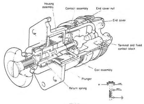
Fig 6.5 Push-in solenoid switch
