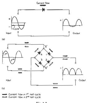
Fig. 3.7 Single-phase rectification (a) Half-wave (b) Full-wave
