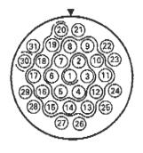
Fig 5.15 Pin/socket sequencing
