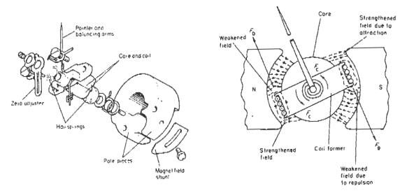
Fig 8.2 Basic form of moving coil indicator
