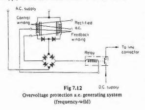
causing its a.c. output to collapse to zero. The relay resets itself and after the fault has been cleared the generator output may be restored and connected to the busbar by carrying out the normal starting cycle.
