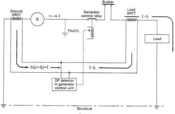
Fig 7.14 -Differential current protection
