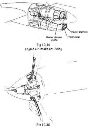
Electrical heater elements - propeller de-icing
