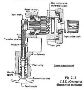
resetting is accomplished by pulling out the reset handle to withdraw the threaded pawl from the input shaft, and allowing the reset spring on the shaft to re-engage the clutch. At the same time, and with the solenoid de-energized, the solenoid nose pin snaps into position in the slot of the pawl.
