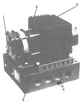
Fig 1.15 Typical single-unit type regulator 1. Armature stop screw 2. Magnet case 3. Heat dissipator 4. Terminal blocks 5. Chassis Fig. 1.16 shows the circuit arrangement of a typica solid-state voltage regulator as employed with the type of alternator shown in Fig. 1.8. Before going into its operation, however, it will be helpful at this stage, to briefly review the primary function and fundamental characteristics of the device known as the transistor.
