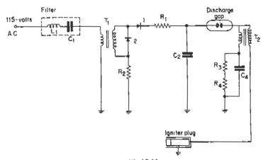
Fig 10.16 High-energy system (a.c. powered)
