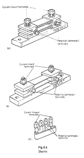
each provided with four terminals. Two of these are of large current-carrying capacity ("current" terminals) for connecting the shunt in series with the main circuit, and two are of smaller size to carry smaller current ("potential" terminals) when connected to the associated ammeter. The unit shown at (a) employs strips of lacquered minalpha spaced from each other to promote a good circulation of air and thus ensure efficient cooling.
