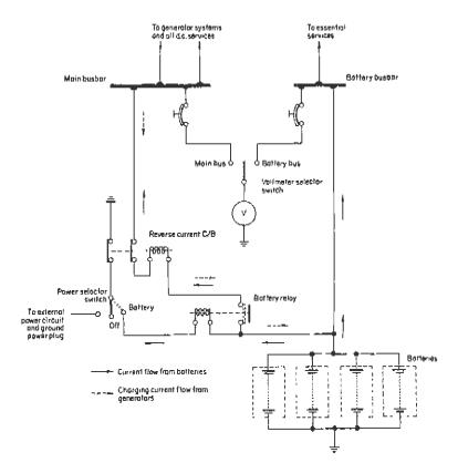
Fig 1.29 Typical battery system circuit
