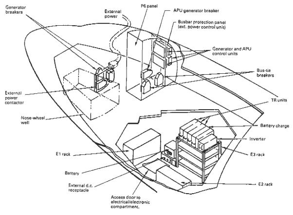
Fig 5.18 Electrical/electronics compartment
