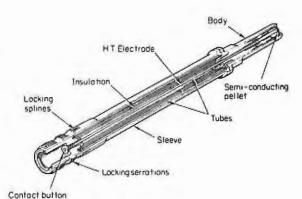
Fig 10.15 High-energy igniter plug
