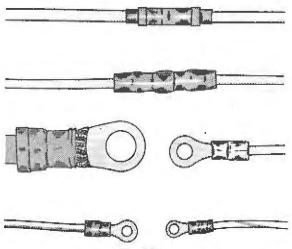
Fig 5.12 Terminals and in-line connectors
