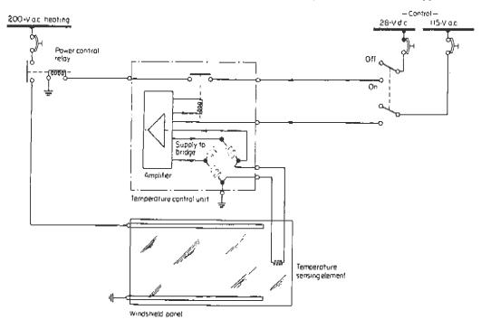
Fig 10.29 Schematic arrangement of windshield anti-icing control system
