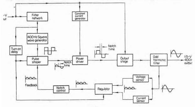
Fig 3.20 Static inverter principle
