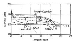
Fig 1.25 Typical discharge rates of lead-acid and nickel-cadmium batteries
