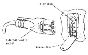
Fig 4.3 External power supply connection
