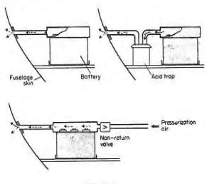
Fig 1.27 Battery venting arrangements
