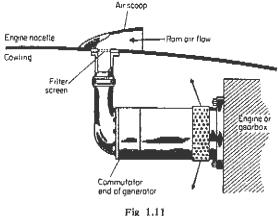
many types of generator have a fan fitted at the drive end of the armature shaft.
