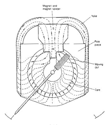
Fig 8.3 Magnet system of a typical long-scale moving coil instrument
