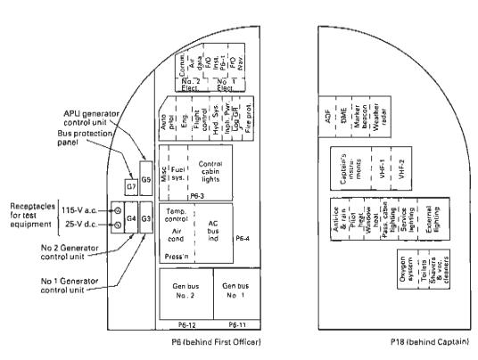
Fig 5.21 Circuit breaker panels (load control centres)
