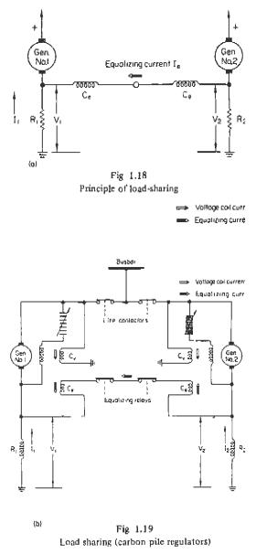
The resistances  $R_1$  and  $R_2$  represent the resistances of the negative sections (interpole windings) of the generators, and under balanced load-sharing conditic the volts drop across each section will be the same,
