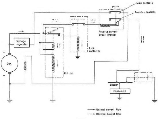
Fig 7.10 Reverse current circuit breaker operation
