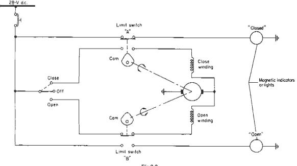
Fig 9.9 Limit switch operation
