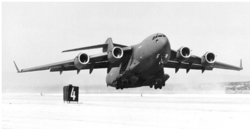
(b) Winglets on a C-17 (USAF Photo)
