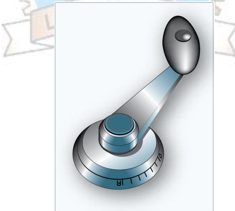
A nose wheel steering tiller located on the flight deck.
