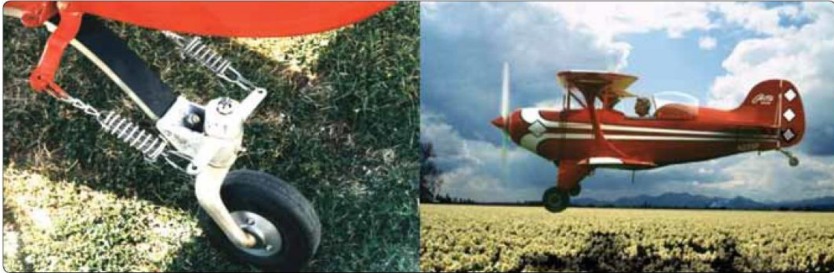
The steerable tail wheel of a Pitts Special.
