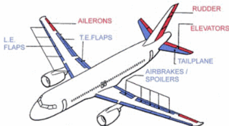
Fig. 8 – Flight control surfaces on airliner
