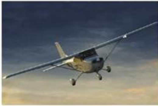
Fixed type of landing gear
