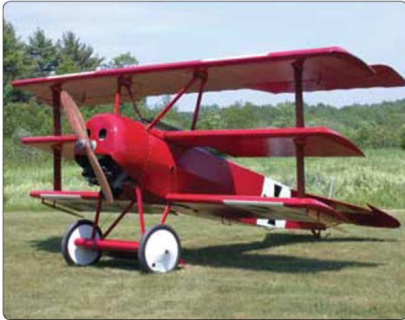
Rigid steel landing gear is used on many early aircraft.
