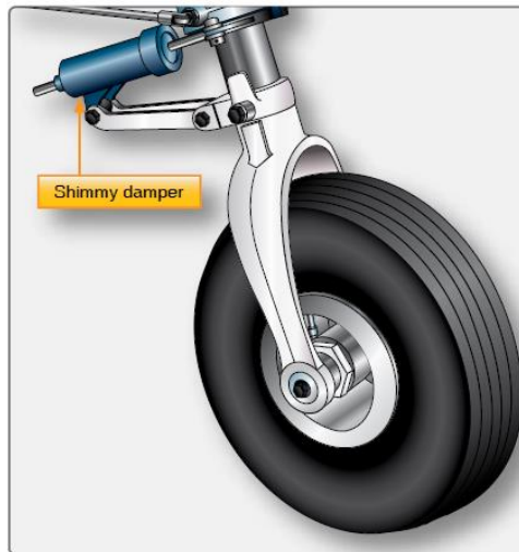
A shimmy damper helps control oscillations of the nose gear.
