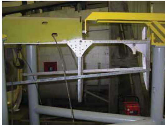
Gussets are used to increase strength.
