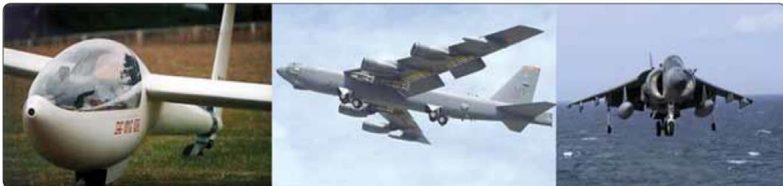
Tandem landing gear along the longitudinal axis of the aircraft permits the use of flexible wings on sailplanes (left) and selects military aircraft like the B-52 (center). The VTOL Harrier (right) has tandem gear with outrigger-type gear.
